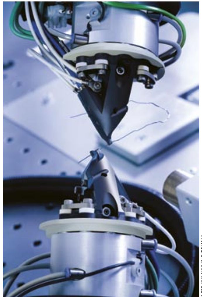
Robotic wire bending of fully customized copper nickel titanium orthodontic wire — a revolutionary merger of high-speed Internet technology, metallurgy and robotics
